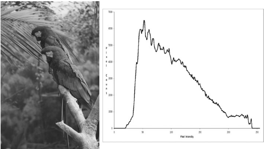
Figure 10-1. Sample grayscale image and its histogram
