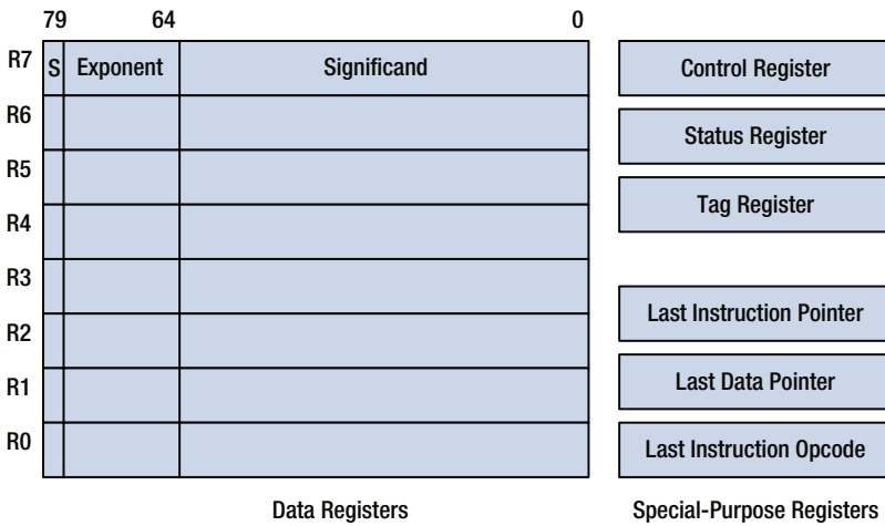
Figure 3-1. X87 FPU core architecture
